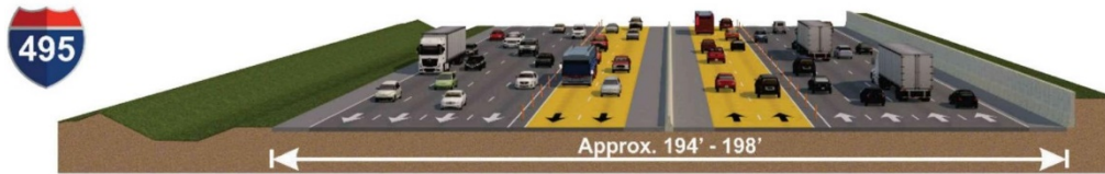
Figure ES-1: Alternative 9 – Phase 1 South Typical Sections (HOT Managed Lanes Shown in Yellow)
